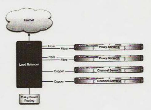
In operation, user TCP port 80 traffic was redirected using Policy Based Routing through a Load Balancer, configured to use TCS (transparent cache switching). This redirected TCP port 80 traffic to the two real proxy-servers.
